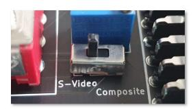
On the V5 and V5.1 versions of the Commodore 128 40/80 Column Video Adapter a secondary switch is added. This switch lets you select the output for the 40 column display. Either Composite (CVBS) or SVideo - Luma/Chroma (Y/C). Best results are generally achieved in SVideo mode. But if you use a third party Scart - HDMI converter, the result is depending on the quality of the converter. Results may vary.
